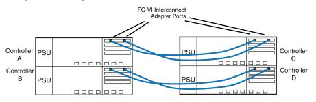
In the previous illustration, one MetroCluster configuration is between Controller A and Controller C.
