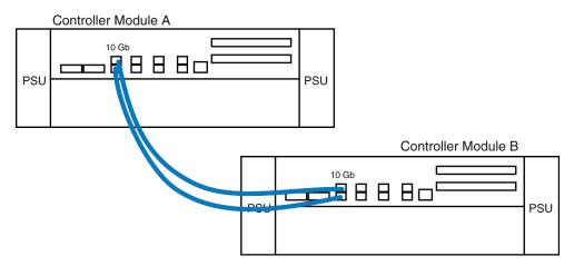
In a dual-chassis HA pair, the controllers are in separate chassis. The HA interconnect is provided by external cabling.
