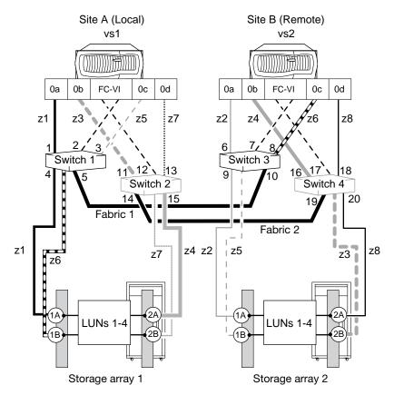
In the sample illustration, four array LUNs are allocated on each storage array for the MetroCluster configuration. LUNs of equal size are provisioned on the storage arrays at both sites, which is a SyncMirror requirement. Each FC initiator port on each gateway has a path to each gateway LUN on the storage arrays. The ports on the storage array are redundant, and are configured as follows:
